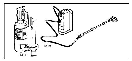
Figure 2-3. Portable Decon Apparatuses
