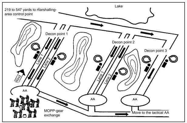
Figure 3-2. Dispersed Operational-Decon Setup
