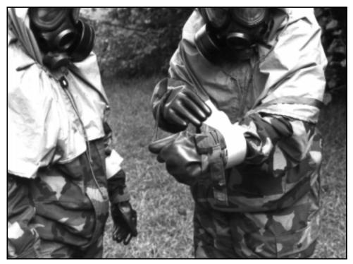
Figure 3-14. Putting on the M9 Detector Paper
