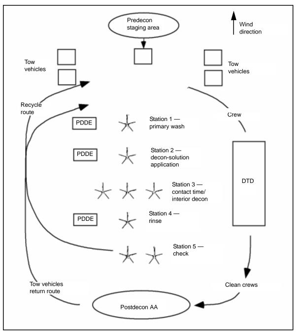
Figure 7-2. Optimum Layout for a DAD Station
